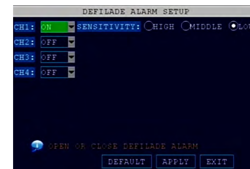
Tamper Alarm Setup
